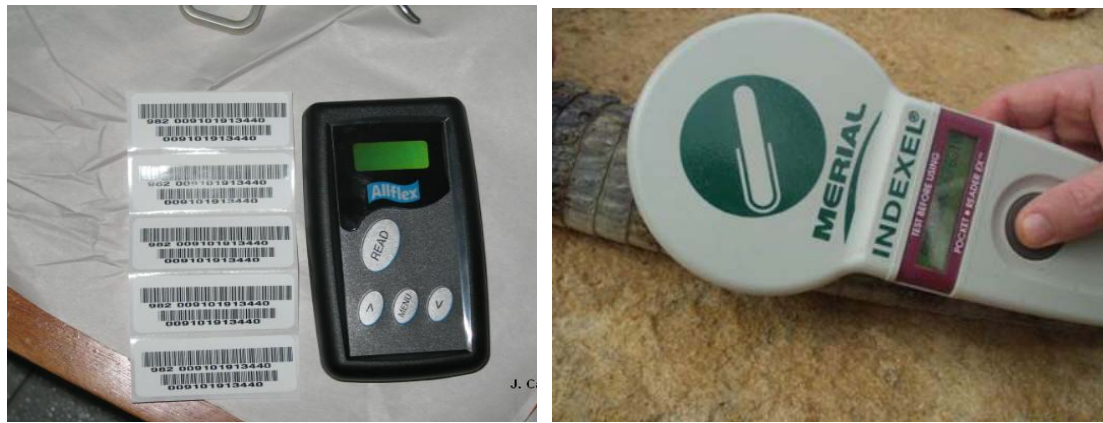
Figure 6. Two types of scanners used to read PIT tags. Photographs: John Calderon (left), Samuel Martin (right).
