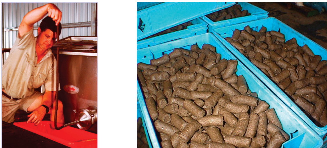
Figure 3. Modified mixer/mincer with pipe die used to produce semi-moist pellets for crocodiles.
